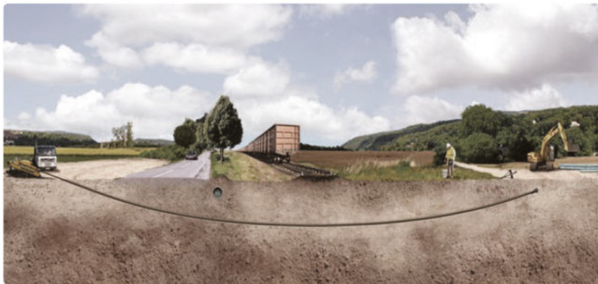
Schematic of horizontal directional drilling (HDD)
